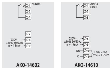
Section of connecting wires for relays contacts should be 2,5 mm<sup>2</sup>.
